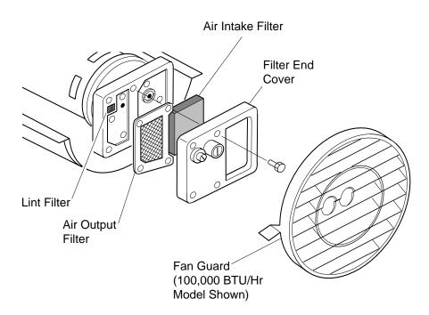
Figure 11 - Air Output, Air Intake, and Lint Filters
